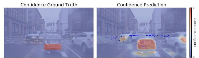
Fig. 1: Radar confidence map comparison. The ground truth is generated by our method, comparing the depth value of the radar point with the ground truth depth map within a selective region.
