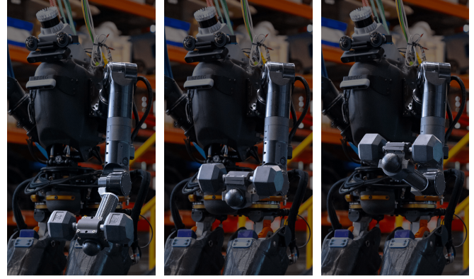
Fig. 6: Nadia curling a 12lb dumbbell after estimating the inertial parameters of the combined dumbbell and forearm link.
