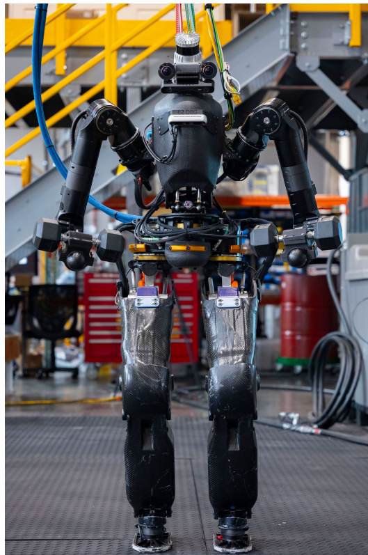
Fig. 1: Our humanoid robot Nadia actively estimating and adapting to 12lb dumbbells attached to the forearms. We use these weights as a proxy for inertially significant manipulation tasks, such as heavy tool use.
