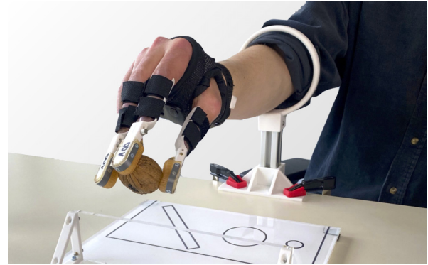
Fig. 1. Passive deformation in soft fingertips is specified through patterns of varying compliance levels across their surface. Performance of different such patterns is compared in human studies. Participants solve various tasks, while operating diverse grippers to which we attach the fingertips.
