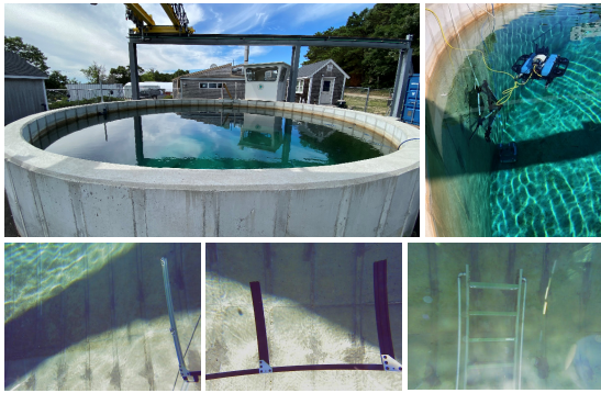
Fig. 5: (Top): The outdoor tank used for data collection exhibits challenging lighting conditions, including reflections (left) and caustics (right). (Bottom): Selected raw (uncalibrated) frames from the vehicle’s monocular camera. These images demonstrate the caustics (ripple lighting effect due to surface waves), reflections, and sudden lighting changes make processing underwater imagery particularly difficult compared to terrestrial scenes. Feature-based methods fail to maintain tracking due to the dynamic textures; our method uses objects instead and proves to be robust to such lighting effects.
