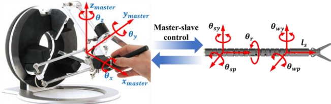
Fig. 8. Mapping relationship in master-slave control.
