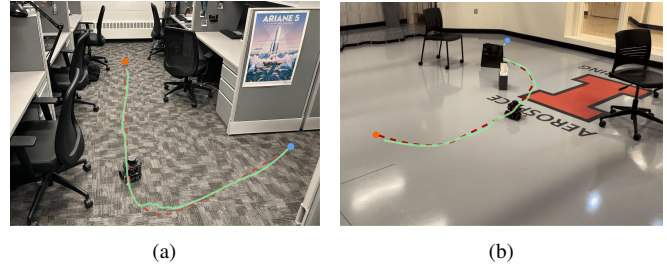
Fig. 1: Performance of ComTraQ-MPC: Fig. (a) depicts ComTraQ-MPC in a known (previously seen during meta-training), trajectory (134 waypoints, active localization budget: 10) and (b) in a previously unseen, longer trajectory (245 waypoints, active localization budget: 20). Start and goal points are marked by blue and orange dots, respectively, with the red dotted line showing the reference trajectory and the green line the ComTraQ-MPC path.
