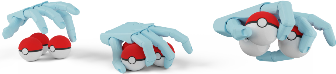
Fig. 1: Our multi-object grasping method, MultiGrasp , drives the Shadow Hand to simultaneously grasp multiple Pokémons.
