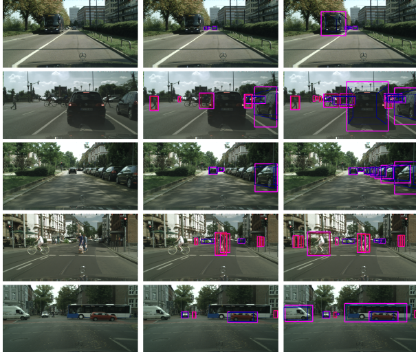
Fig. 5: The qualitative results on the Cityscapes dataset. The leftmost column contains the original images, the middle column displays the zero-shot results, and the rightmost column shows the results obtained using our method. The pink boxes represent 2D detection results.
