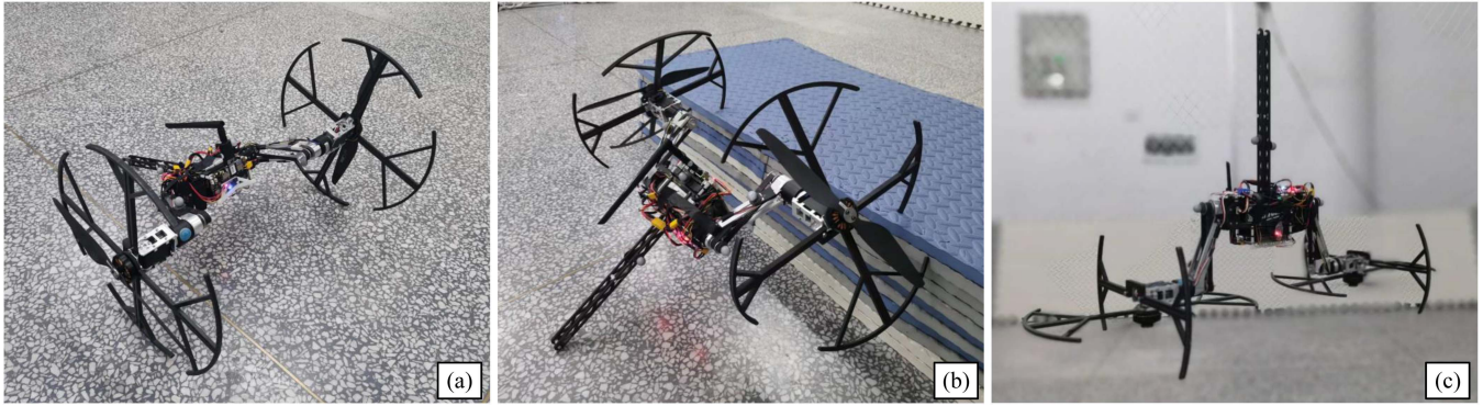
Fig. 1. Morphable terrestrial-aerial robot. (a) Configuration of rolling mode. (b) Configuration of climbing mode. (c) Configuration of flying mode.
