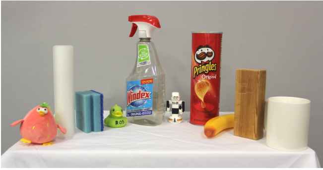
Fig. 5: Evaluation objects: Plush Toy, Rubber Mat, Sponge, Duck, Spray, TIAGo, Pringles, Banana, Wood, and Mug. Ordered by increasing stiffness from left to right.
