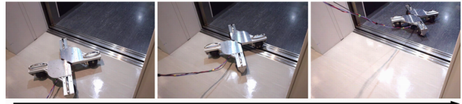
Fig. 15. Overcoming the gap in the elevator. We confirmed that stability is maintained during forward, backward, lateral, diagonal, and turning movements.
