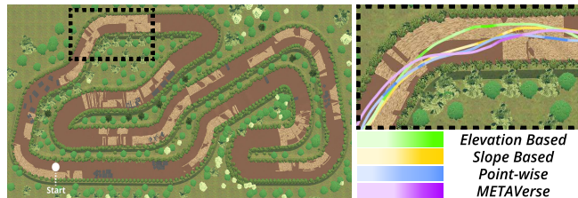
Fig. 5: (Left) The off-road race track for the navigation experiment (Q2). (Right) Vehicle trajectories taken by employing various traversability maps. We observe that METAverse can navigate through relatively safer trajectories by accurately identifying nuanced traversability.
