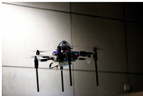
Fig. 1. Our hexacopter, as designed in [6], is transitioning from a well-lit environment to a dark area, where the accuracy of VIO degrades due to lack of visual features.
