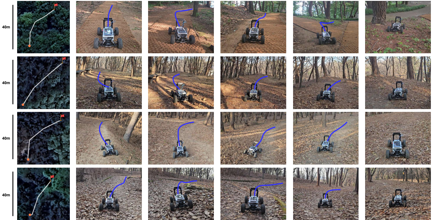
Fig. 7. We show the navigation results of our proposed navigation system. While driving in unpaved outdoor environments, our navigation system performed path planning and execution. The first environment is the place where we collected data. The second, third, and fourth are out-of-distribution environments where we did not collect data. The blue lines show the planned trajectories. We arrived at the goal position without failure.
