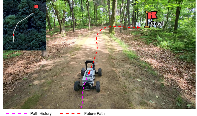
Fig. 1. The wheeled robot platform, Raicart , adeptly navigates through unpaved outdoor terrain. The environment is a straw blanket on a dirt road. Raicart navigates this challenging course without explicit object segmentation. The proposed navigation system finds a path that minimizes bumpiness and oscillation in orientation.
