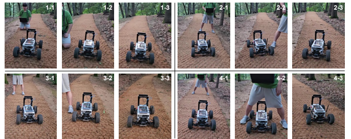
Fig. 9. Results of obstacle avoidance. When a human is on the side of the straw blanket, the robot navigates to the other side, preventing bumpy events. The robot did not get out of the straw blanket in this evasive maneuver. When both sides are blocked, the robot chooses a path to pass through the legs.
