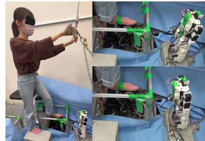
Fig. 7. Operating experiments with foot control. (Above: tilt to over 5[deg]. Below: return to 0[deg].)
