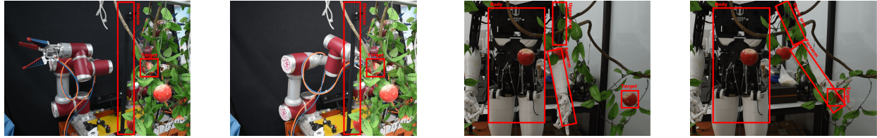
(a) Initial and end Kuka arm positions reaching the target while avoiding the cylinder obstacle in-between.
