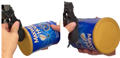
Fig. 9: Demonstration of data collection process. We collect a real-world dataset by pressing the tactile sensor-equipped fingertip on flat surfaces (left) and curved surfaces (right).
