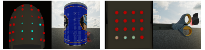
Fig. 4: Illustration of data collection using NVIDIA Isaac Sim simulator. The figure shows the curved fingertip sensor (left) and the 4 \times 4 flat pad sensor (right), respectively.
