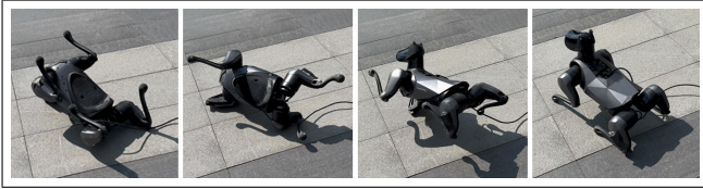
Fig. 5: Recovering from a failed jumping. The estimated robot height from the estimator is used as one of the conditions for triggering the reset policy.
