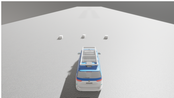
Fig. 3. A CARLA simulation environment showing three cubic calibration targets with edges of 0.5 meters in close proximity. The digital twin of the EDGAR [26] research vehicle is placed at the origin of the world.
