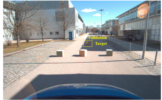
Fig. 4. Real-world experimental setup with three cubic calibration targets with edges of 0.5 m placed on a regular road. Another target is placed at a distance of about 16 m.
