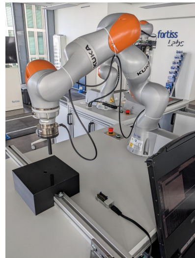
Fig. 3: Demonstrator setup with a KUKA IIWA 7 R800 robot and attached cylindrical peg, black target box with hole, and Kapoho Bay containing two Loihi chips (on the tabletop).
