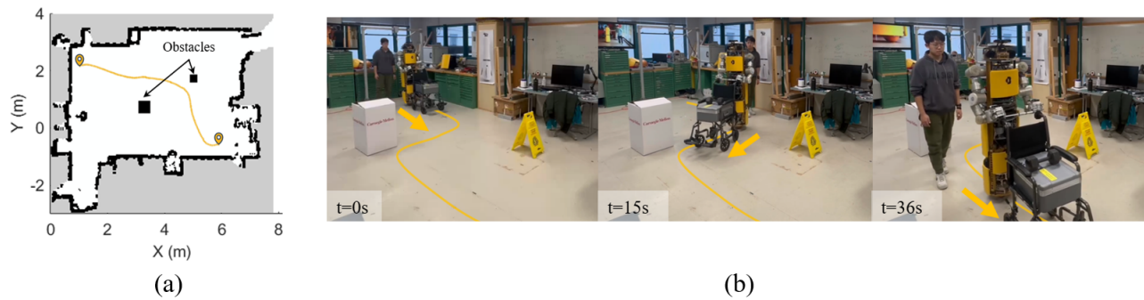
Fig. 10. Navigation across lab with predefined obstacles. (a) Map with pre-defined obstacles. The markers indicate the start position (left marker) and goal position (right marker), and the yellow line shows the actual trajectory of the ballbot. (b) Time-lapse picture of the experiment. Yellow arrow indicates ballbot's velocity direction.
