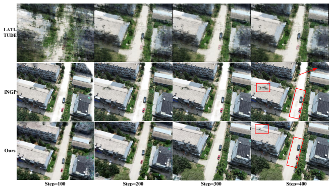
Fig. 3. Frame2Model registration results: the LATITUDE[27] experiences registration failure due to aliasing, resulting in confusion in the merged observation and rendering images. While the iNGP[11] shows notable accuracy improvements, noticeable floating artifacts in the highlighted area are observed, potentially inducing registration errors. Ours effectively avoids aliasing, ensuring superior rendering quality and registration accuracy.
