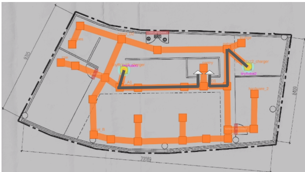
Fig. 9. Example of simulated world. The arrows show requested trajectory in an example scenario. The reservation system would re-order the requests such that no two robots would conflict with each other for use of the pantry.
