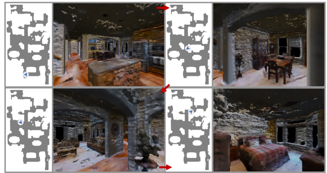
Fig. 5: Navigating in the Habitat simulator: the underlying mesh was extracted from the trained NeRF, Ours (cov) . Rendering quality and the generated BEV map are correct, as are free navigable space and collision handling. Temporal order indicated by \rightarrow .
