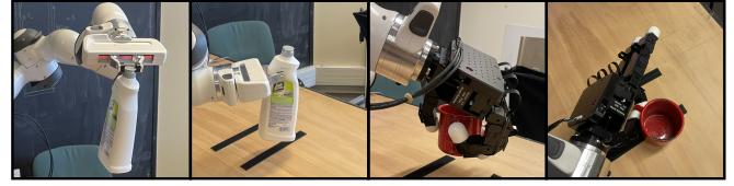
Fig. 8. Examples of transferred grasps. The proposed method generates diverse grasp poses that are robust in the physical world.
