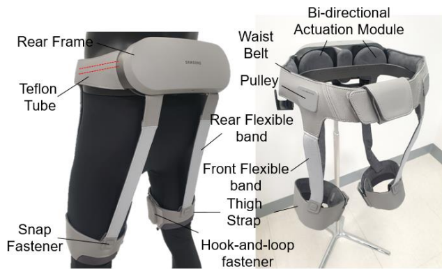
Fig. 2. Overview of the mechanical design
