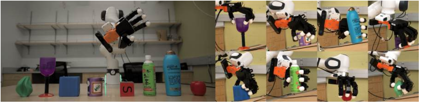
Fig. 3: Left. Hardware setup. We synthesized grasps on eight objects for an Allegro hand mounted on a Franka Research 3. From left to right: 3D-printed part, goblet, box, mug, cube, bottle, conditioner, and apple. We employed an eye-in-hand setup with a Zed camera to capture images used to train a NeRF prior to grasping. Only monocular RGB was used. Right. Representative FRoGGeR-synthesized grasps.
