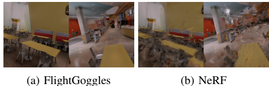
Fig. 2: (a) Images captured in the Flightgoggles simulation environment [18]. (b) Images rendered through nerfstudio [29]. The images exhibit significant differences from the originals, primarily due to artifacts caused by the sparse density of training data.
