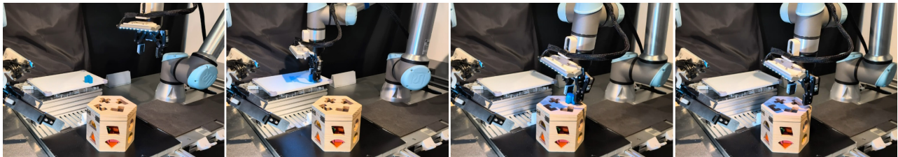
Fig. 6: Single-arm Picking & Insertion : The task consists of picking up a toy wooden peg and inserting it into its corresponding hole in a wooden box. A proper grasp is required to facilitate the alignment of the peg with the hole. During demonstrations, the demonstrator utilizes a medium stiffness mode for general manipulation and switches to a low stiffness mode for the insertion phase that involves physical contact. The peg is placed at the edge of the whiteboard with a random rotation of about \pm 15^\circ . The wooden box's position is not fixed, so the robot can move it during the peg insertion. 30 demonstrations were collected for this task.
