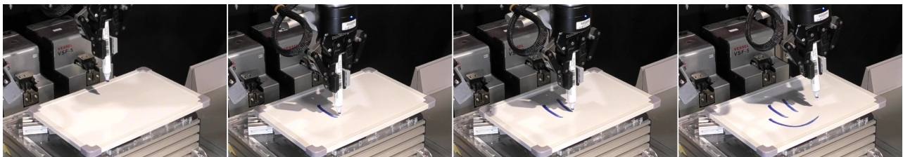
Fig. 8: Single-arm Drawing : The goal is to draw a simple emoji smile on a whiteboard. The task starts with the robot already grasping a pen. The robot must write three parts of a face while keeping a consistent force while in contact. This task is interesting in that it requires frequent switching between in-contact writing and free motion. It also requires careful coordination of the positional relationship between each part of the smile. During demonstrations, the demonstrator employs a medium stiffness mode for the free motion between drawing stages and transitions to a low stiffness mode to apply force during the in-contact drawing. 20 demonstrations were collected for this task.
