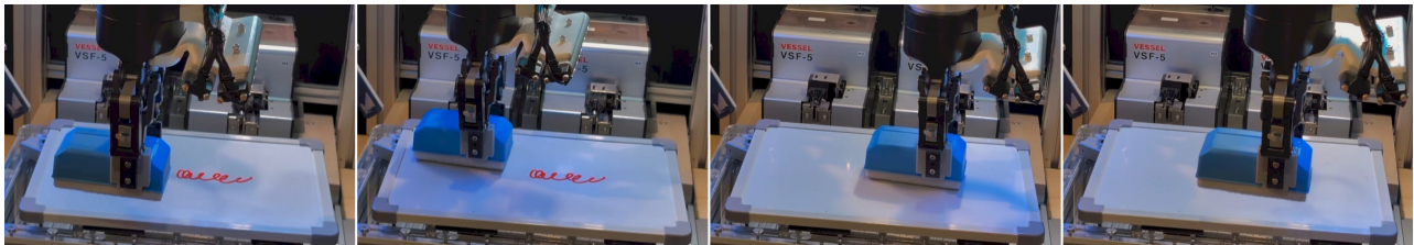
Fig. 7: Single-arm Wiping : The goal is to wipe marks on a whiteboard. The task starts with the robot already holding the eraser. During demonstrations, the demonstrator begins with a medium stiffness mode to approach and then switches to a low stiffness mode to apply force to the whiteboard. The task requires applying sufficient contact force to the board during the wiping motion. The task starts with a random mark drawn in an area of \pm 5 cm from the center of the board. 20 demonstrations were collected for this task.
