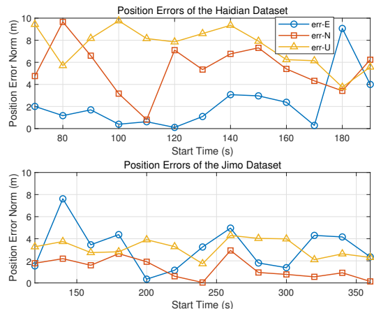
Fig. 6: Position errors in different directions, where ‘err-E(N/U)’ denotes the error in the east (north/up) direction.
