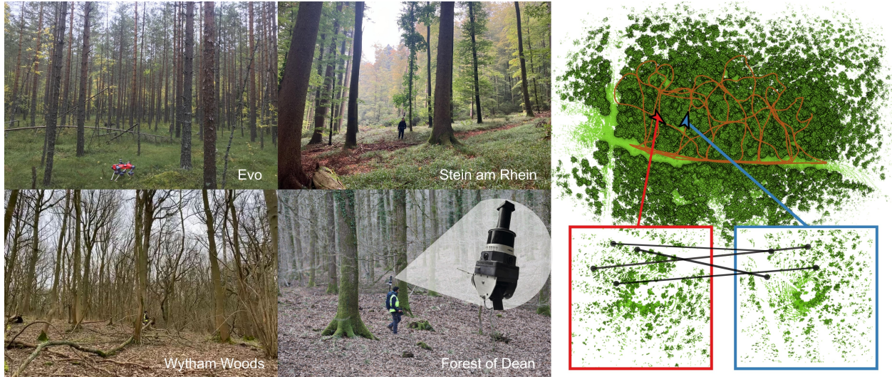
Fig. 1: In this work we evaluated LiDAR-based place recognition in dense forest environments. Left: Four different forests test sites: Evo (Finland) and Stein am Rhein (Switzerland) are coniferous forests, and Wytham Woods and Forest of Dean (UK) are deciduous. Data collection primarily utilized backpack-mounted LiDAR systems, with additional relocalization experiments conducted using a LiDAR-equipped legged robot. Right: Illustration of loop closure detection within a deeply forested area, with offset distance of 11.2 m and orientation of 96^\circ between the matched scans. The black dots indicate some corresponding locations in the two point clouds for illustration purpose.
