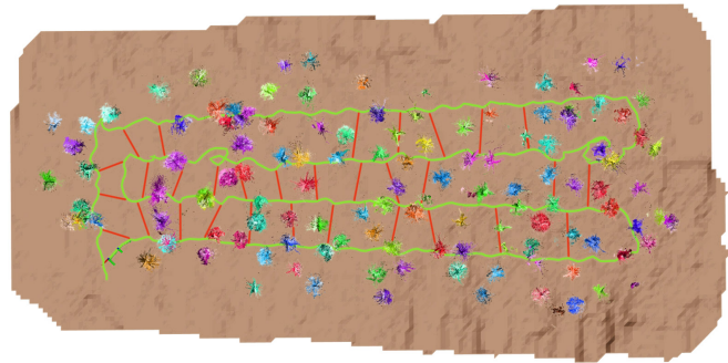
Fig. 11: Fully autonomous mission through a plot of the Forest of Dean with the ANYmal quadruped autonomously navigating the forest following a lawn-mower pattern. On board the Mobile Robot, our pipeline created an online forest inventory which was visualized for the operators in real-time. Note the pose graph (green) being corrected using loop closures (red).
