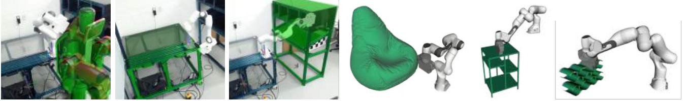
Fig. 5: Environmental objects used in experiments: Baxter (real), table (sim/real), shelf (sim/real), beanbag (sim), nightstand (sim), winerack (sim). The green overlays are the objects' mesh models, displayed relative to the robot's base frame based on the robot's self-calibrated pose.
