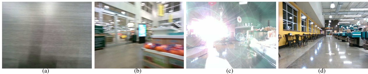
Fig. 2. Representative images from our datasets: (a) nearly textureless area, (b) severe motion blur, (c) bright sunlight, and (d) moving light glare.
