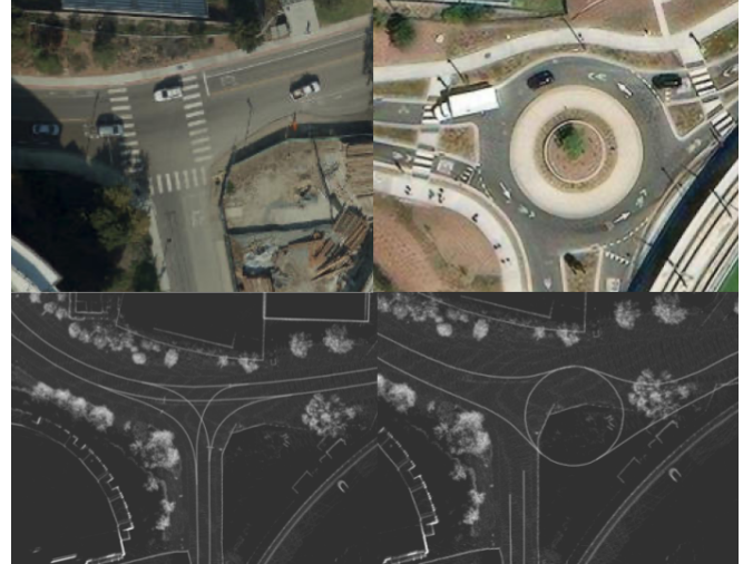
Fig. 1. Spatial Evolution of a road network at the UC San Diego Campus in both satellite image [6] and vectorized centerline map [7]. The left side of the figure depicts the area prior to 2021, while the right side presents the current state of the road network. Below the satellite image, the corresponding vector map from the respective time period is displayed.
