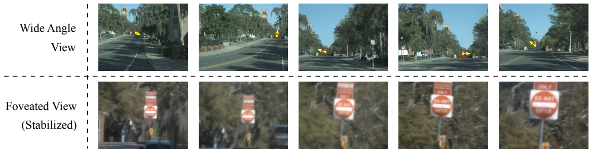
(c) Stabilization on a traffic sign with the camera mounted on a vehicle driving towards it. The sign stays in the center of fovea FOV even when driving over speed bumps.
