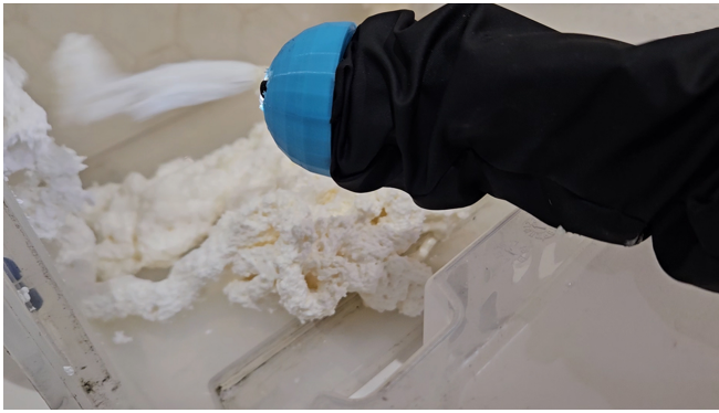
Fig. 8. Hybrid robot showcasing adaptability in simulating scenario 3, employing an expanding foam application to effectively cover the walls of the glove box.
