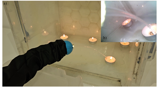
Fig. 7. a) Hybrid robot demonstrating its versatility in simulating scenario 1, effectively extinguishing a candle by employing a water-spraying mechanism. b) A POV view of the target, using the built in tip mounted micro camera.
