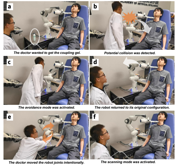
Fig. 7. Snapshots of experiment 2: (a) t = 2.5 s. The robot was performing the scanning task. (b) t = 5.2 s. The doctor wanted to put the coupling gel on the back of the robot. The robot detected the potential collision and entered Avoiding Mode . (c) t = 7.0 s. The Avoiding Mode enabled the doctor to the place conveniently. (d) t = 10.0 s. The robot returned to its original configuration for scanning. (e) t = 19.0 s. The doctor contacted the robot in the null space, the Contacting Mode was activated, and the error and force of the end effector main task were unaffected. (f) t = 25.0 s. The Scanning Mode was activated.
