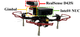
Fig. 5: The customized quadrotor used in real world experiments.
