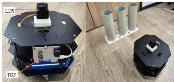
Fig. 5. Calibration of the experimental platform. ToF depth camera and LDS sensor mounted on a mobile robot.
