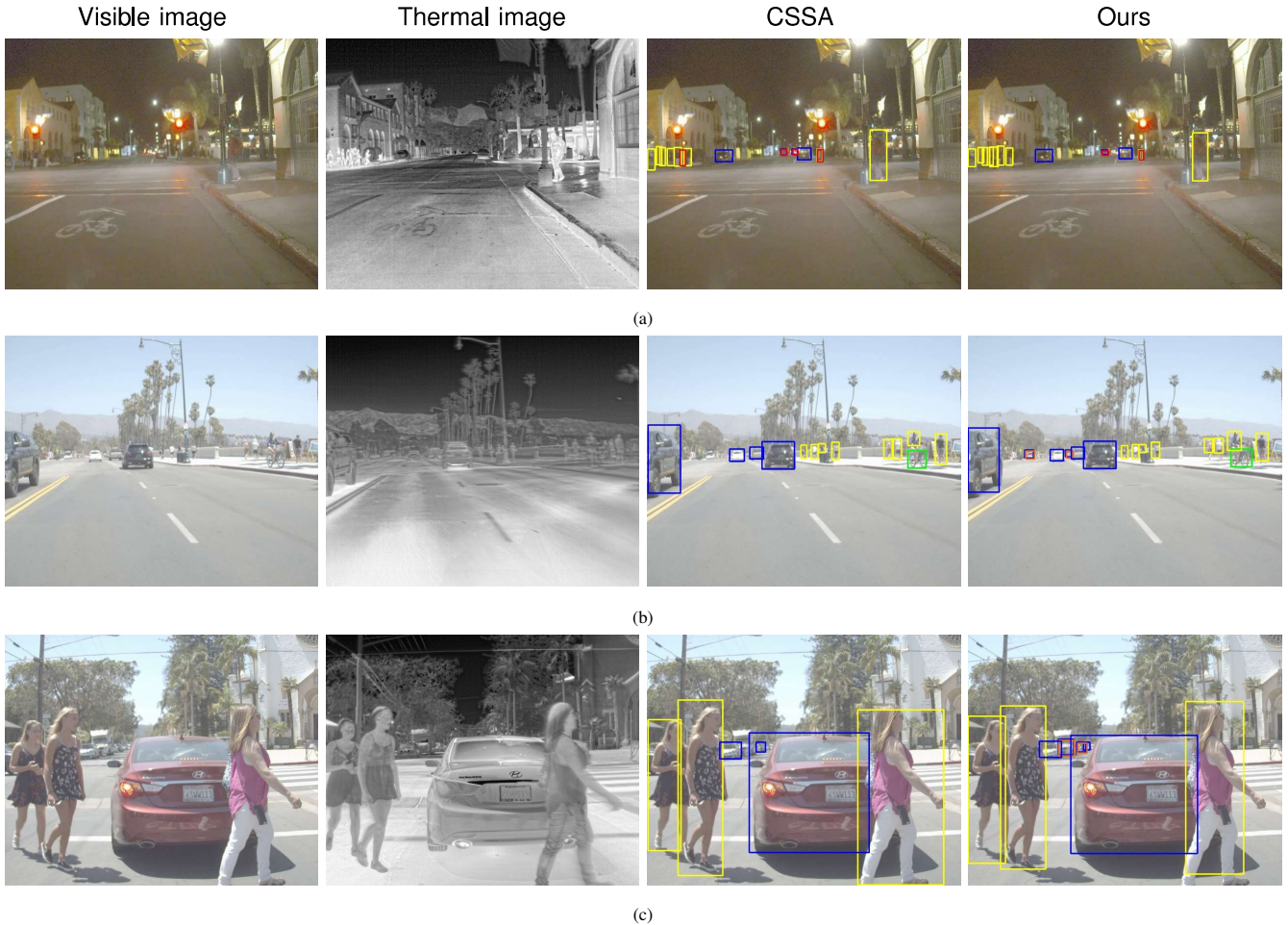
Fig. 5. Visualization of results with the optimal contrast model CSSA [37]. Each row is a sample. The person, car, and bicycle are marked with bounding boxes in blue, yellow, and green. The red box is used to mark detection errors (false alarms/missed detections), and orange box is used to mark objects that are not in labels but are actually present and successfully detected in the image.
