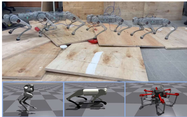
Fig. 1: (Top) Our position-assisted, torque-based policy, can successfully help the robot navigate real-life uneven terrain, despite having been trained on flat ground without any external force disturbances. (Bottom) Our torque-based velocity tracking policies for Agility-Cassie (left), Unitree-Go1 (middle), and Hebi-Daisy (right), achieve high-quality gaits within just 25 minutes of wall-clock time. 4
