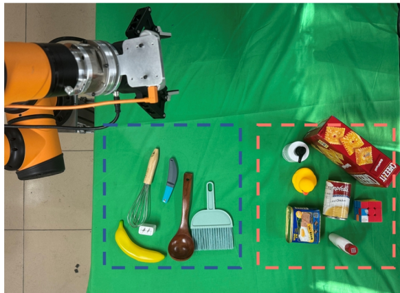
Fig. 7. Robot and object settings in real-world experiment: the blue box is used for testing small-scale grasps, while the red box contains objects for testing medium to large-scale grasps.
