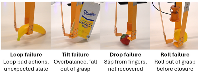
Fig. 7. The four most common failure modes observed during testing.
