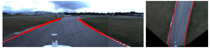
Fig. 2. Example of output resulting from the road line markings extraction pipeline: on the left, the points reprojected (using the homography matrix) onto the image plane; on the right, the same points in BEV space.
