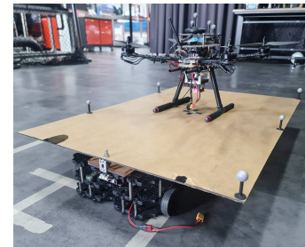
Fig. 7: The quadrotor platform and the TurtleBot -based moving landing platform for real-world experiments.
