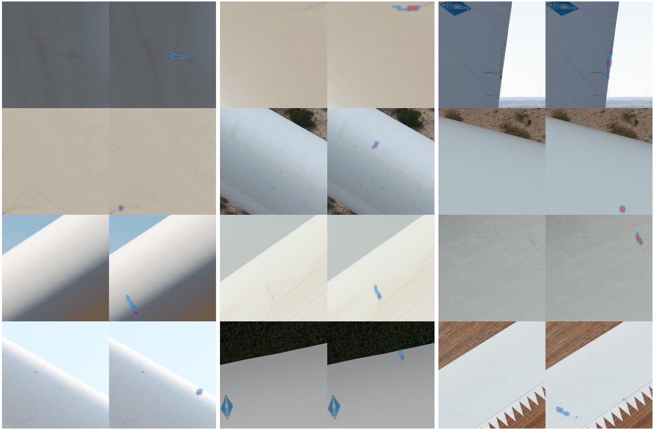
Fig. 4: Sample Crack Detection Region Proposals using the GradCAM method [38] . Our pipeline provides region proposals to a human analyst who then reviews and further diagnoses barely-visible surface hairline cracks for severity categorization and repair recommendations. We first compute the GradCAM attributions w.r.t the crack detection class model output. We then post-process the attribution heatmap using the normalize and polygonize operations.
