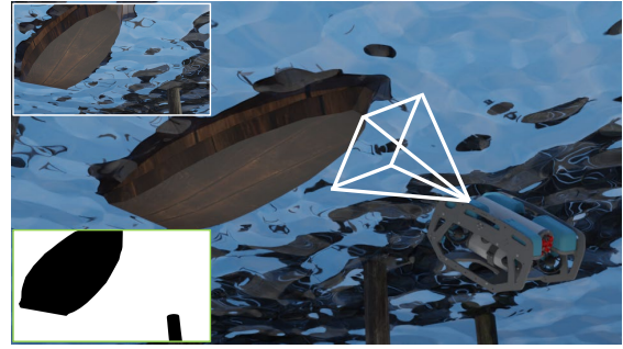
Fig. 2: BlueROV collecting data for our synthetic dataset in AquaSim . The inset shows a sample image captured from the camera on a BlueROV. The top left displays the feed from a front-facing RGB camera, while the bottom left shows the real image’s corresponding ground truth masks.
