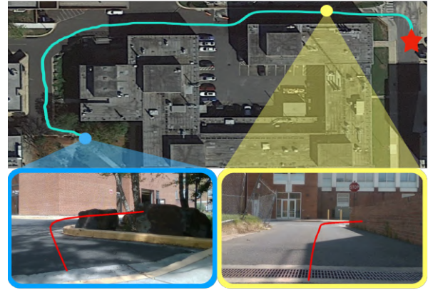
Fig. 1: DTG generates trajectories in traversable areas with the shortest travel distance to the target (red star). The blue and yellow boxes show the efficacy of the generated trajectories in scenarios including bushes and buildings.
