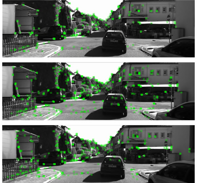
Fig. 4: Processing results for dynamic objects. From top to bottom, they are BE-SLAM, ORB-SLAM2, DynaSLAM.
